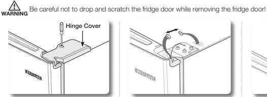
1. After removing the screw, remove the upper Hinge Cover.
